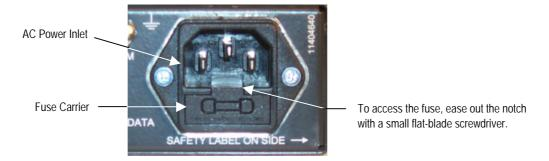
Figure 6.2: Fuse Carrier
